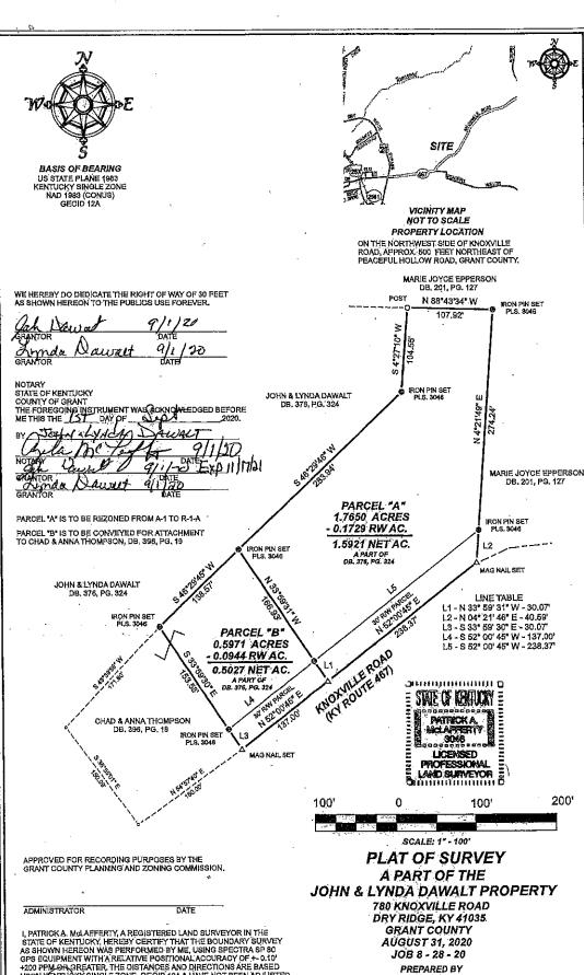
I, PATRICK A. McLAFFERTY, A REGISTERED LAND SURVEYOR IN THE STATE OF KENTUCKY, HEREBY CERTIFY THAT THE BOUNDARY SURVEY AS SHOWN HEREDN WAS PERFORMED BY ME, USING SPECTRA AS 9 80 GPS EQUIPMENT WITH A RELATIVE POSITIONAL ACCURACY OF 1-0.10' +200 PPM-OR GREATER, THE DISTANCES AND DIRECTIONS ARE BASED UPON KENTUCKY SINGLE ZONE, GEÖID 12A & HAVE NOT BEEN ADJUSTED. THIS SURVEY MEETS OR EXCEEDS THE MINIMUM STANDARDS FOR A RURAL SURVEY AND COMPLIES WITH 201 KAR 18:150.
